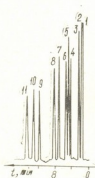
Fig. 4. The separation of alkanes and isomers of disubstituted benzene on the deactivated column 15.5 m x 0.3 mm with phase I. Column temperature 50° (supercooled mesophase), carrier gas—helium 23.5 cm/s, make up gas—nitrogen 40 cm 3 /min. Peaks: hexane (1), heptane (2), octane (3), m-xylene (4), p-xylene (5), o-xylene (6), m-ethyltoluene (7), p- and o-ethyltoluene (8), m-diethylbenzene (9), o-diethylbenzene (10), p-diethylbenzene (11).
