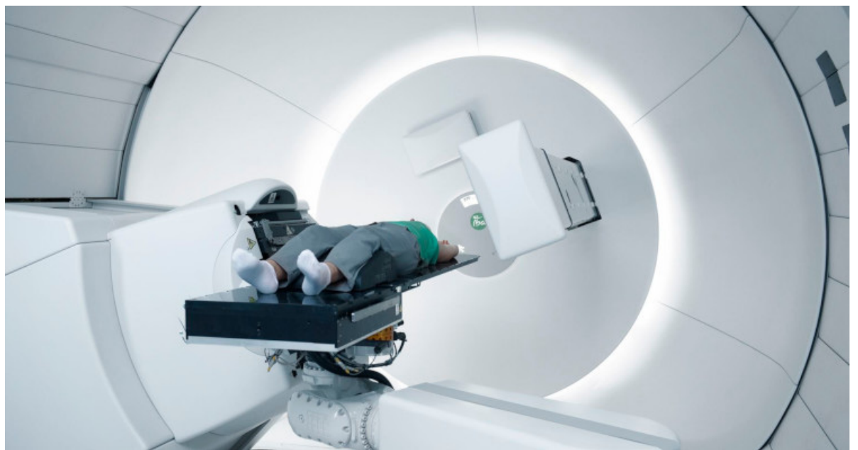
Hadron therapy uses beams of charged particles like protons, carbon ions and other ions to kill tumor tissue. Unlike photons or electrons, which release energy along the length of their path, the charged particles deliver most of their damaging energy in one burst inside the tumor.
