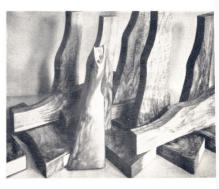
STAGES IN the carving and attachment of the wood stock to the action. Above, the locks are being cut in.
