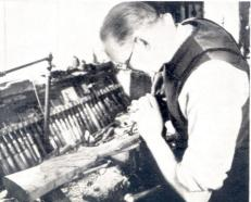
STRIPPING AND POLISH-ING the steelwork preparatory to the final process of engraving.
