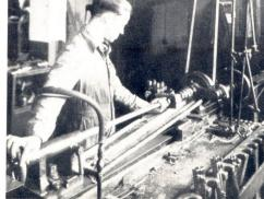
CHAMBERING the barrels. This is a very important stage, as gas tightness and the fit of the cartridge in the chamber both depend entirely on the accuracy and smoothness of the cutting. Though the aid of the machine has been called in as far as possible, individual skill and workmanship are still depended on to turn out the gun of to-day.
