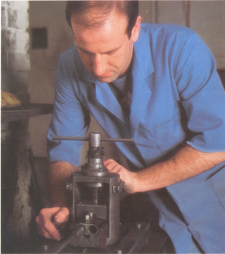
Lapping the bore of a pair of shot gun barrels.
