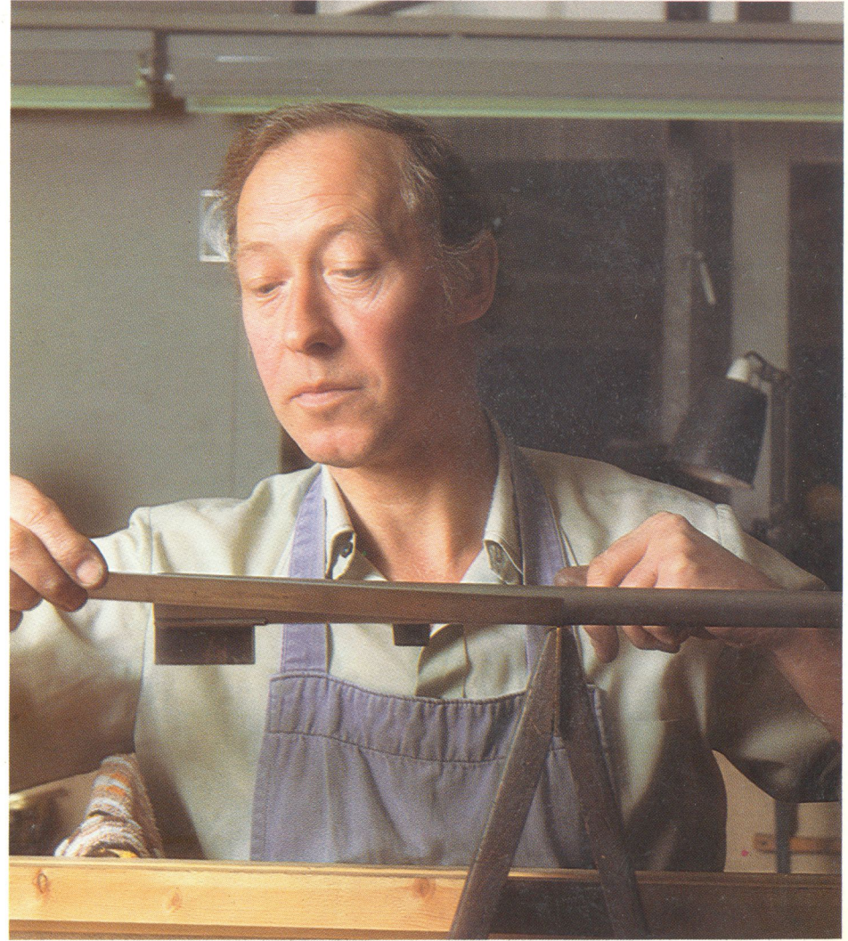
Checking a pair of rifle barrels for weight and balance.
