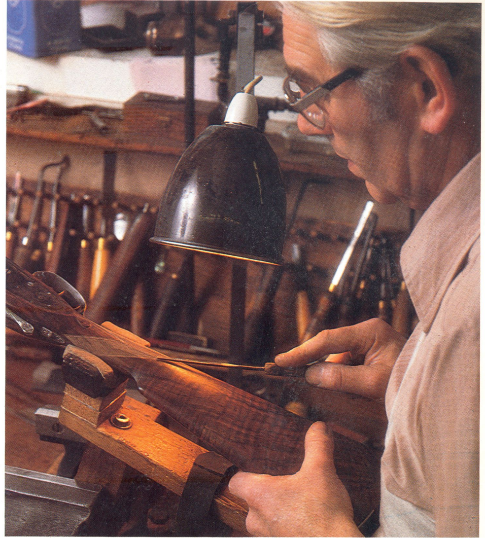
Chequering the stock. Purdey chequering is worked to approximately twenty-four lines to the inch.
