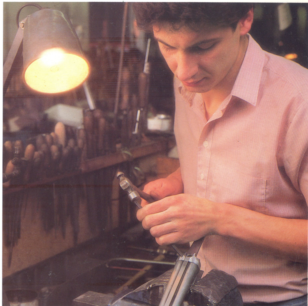
Chasing the fences on a side-by-side gun.
