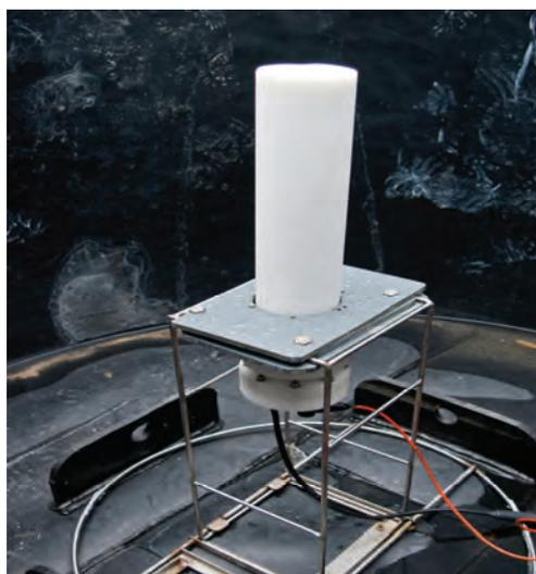
*Figure 1. The underwater gamma-ray spectrometer of Hellenic Center for Marine Research named KATERINA into the artificial tank before the fulfilling with groundwater from the aquifer of Grand Sasso.*
