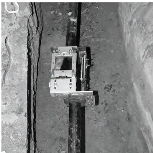
Fig. 7. A photograph of monitoring point B6. The left-lateral displacement of steel holders is obvious (after Dobrev, 2011).
