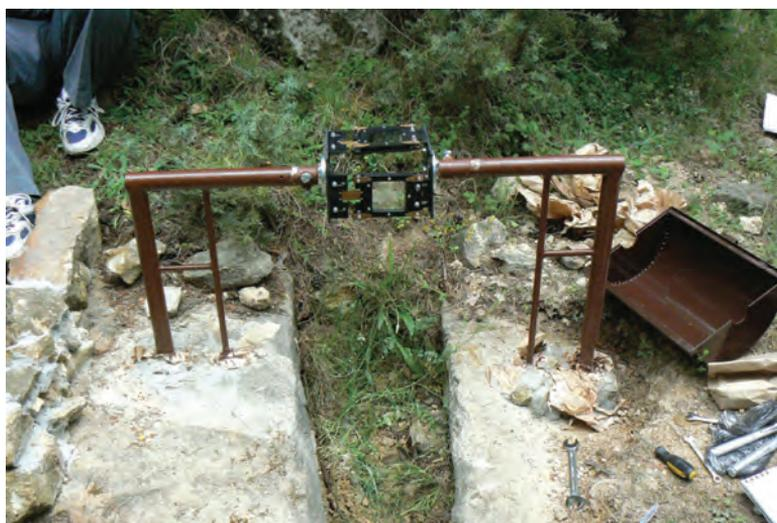
Figure 9. The newest extensometric point J13 near Jaladovo Village installed in 2010 (Krastanov et al., 2010)
