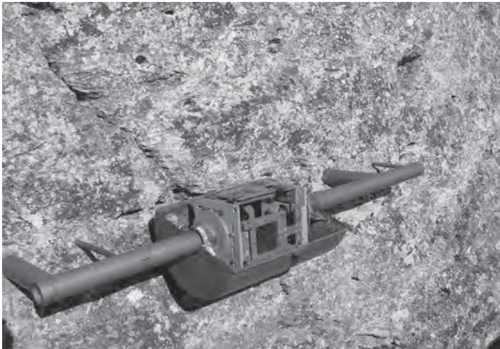
Figure 1. A view of 3D extensometer TM71 (Madara monitoring site M8)
