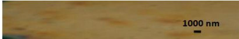
**Figure 2.** Microstructure of  $h \approx 200 \text{ nm}$  thick SiO<sub>2</sub>+TiO<sub>2</sub>+ZrO<sub>2</sub>+Au<sub>0.03</sub> film on Si(100) surface.
