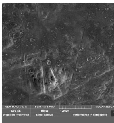
**Figure 2.** SEM image of base glass surface.
