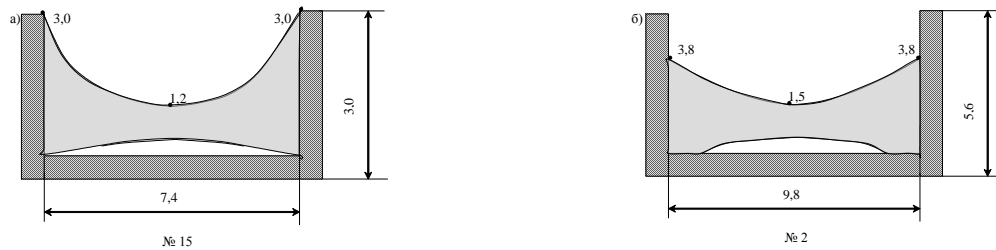
Figure 14. “Critical” cross-sections: a) of blocks B-6 with Q = 0.72 l/s and b) of long-dimensional blocks with Q = 1,44 l/s (dimensions are given in cm) [results their own research]
