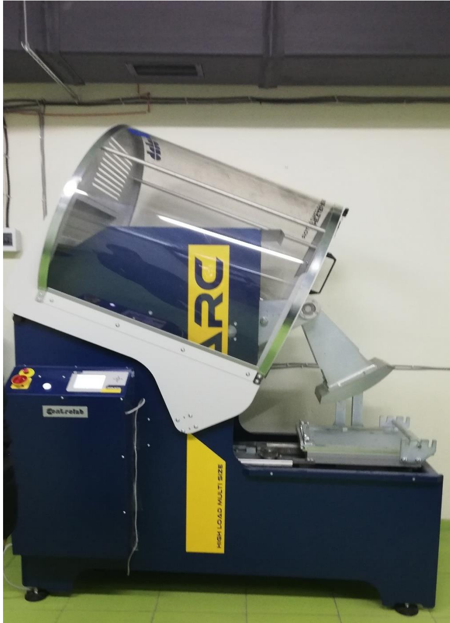
სურ. 21 Heated asphalt roller compactor
