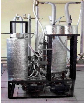
Figure 5. Experimental installation for combined microwave and supercritical CO 2 fluid extraction
