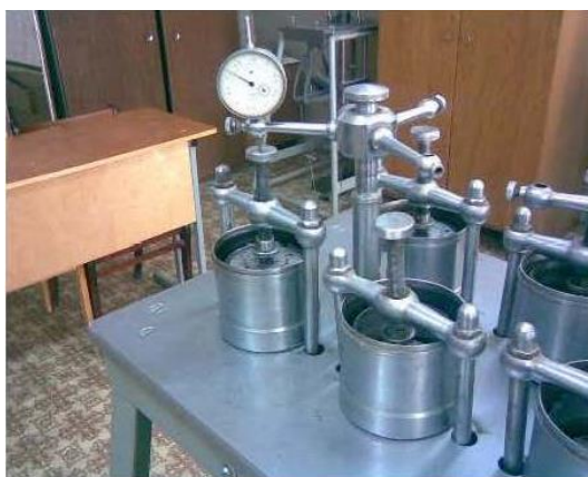
Fig. 1. The compression device and its scheme
