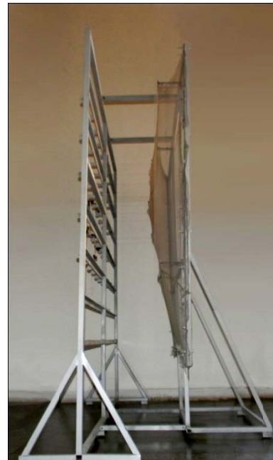
Fig. 3.6. Test bench 1 – Stand framework; 3 – Reflecting Mesh; 6 – load points
