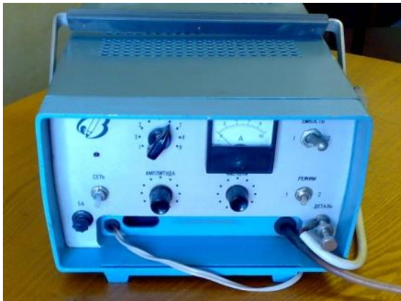
Fig.2. Device for electrospark doping
