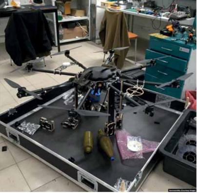
The commercially popular DJI drones, An R18 drone with munitions. Photo from Aerorozvidka NGO
