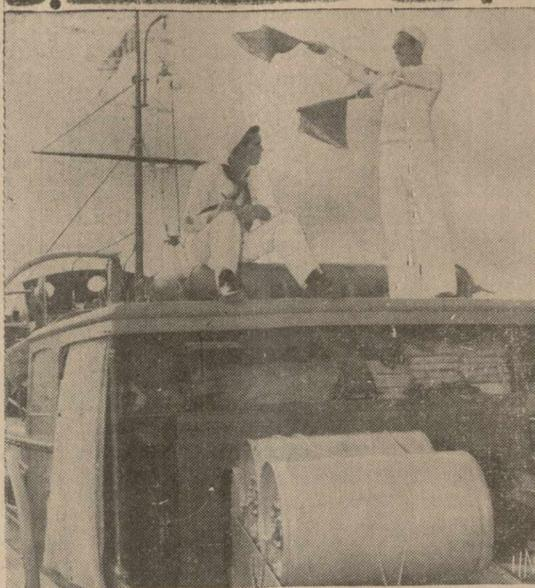
Members of the U. S. Naval Sub-Chaser School at Miami, Fla., are shown testing their ability to exchange signals aboard a modern sub-chaser. This method of "talking" is very important in modern warfare, as the use of the radio would give away the ship's position to the enemy. Note the "ash cans" (depth charges) in the foreground.
