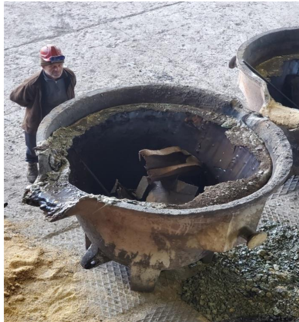
Fig.1. Placement of steel scrap in the ladle
