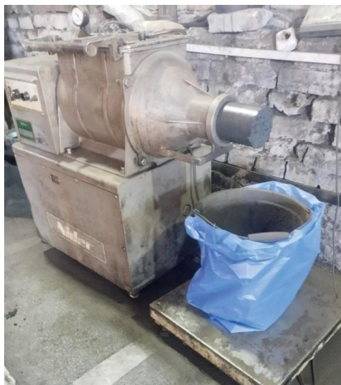
Fig. 3. A kneading apparatus (Shimpo NVS-07) for making paste
