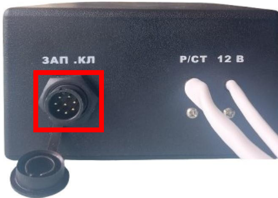
Figure 6. Key loading into the HF encryptor is performed through an 8-pin connector
