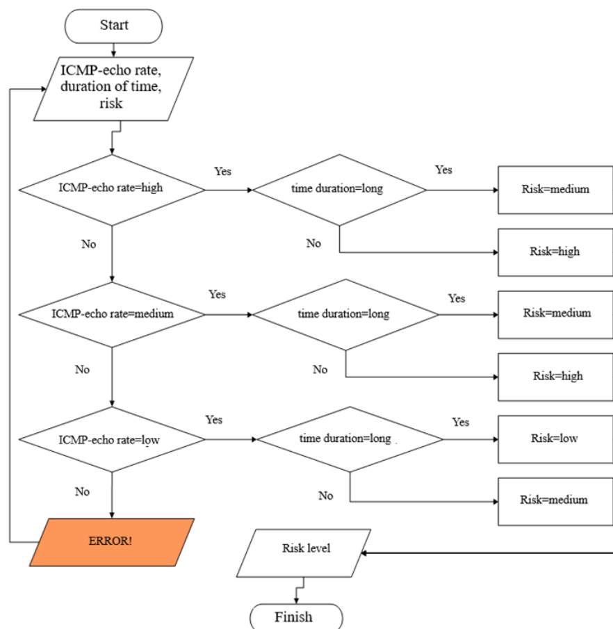
Figure 2. Block diagram of packet filtering rule algorithm (first level: fuzzy filtering)
