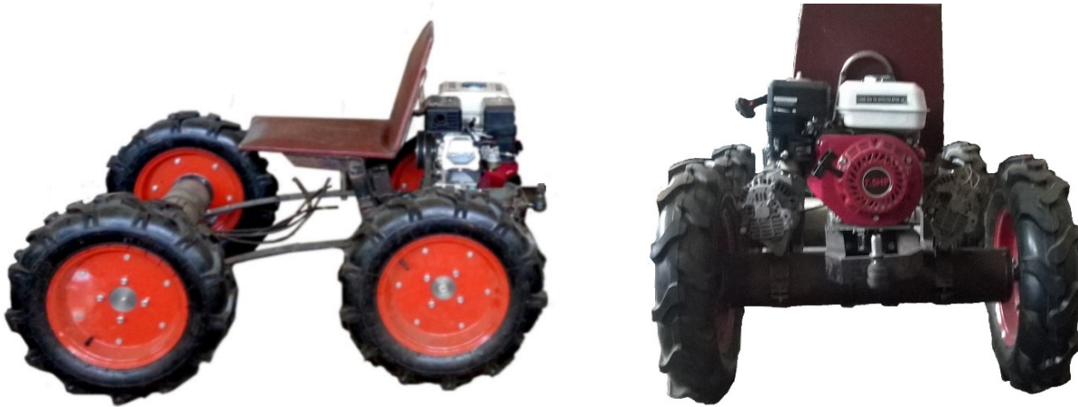
Fig. 2. Acting physical model of the hybrid type mini-mobile machine.
