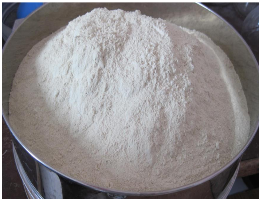
Fig. 3. Photo of AgI/nanosilica powdery reagent (LN-212).
