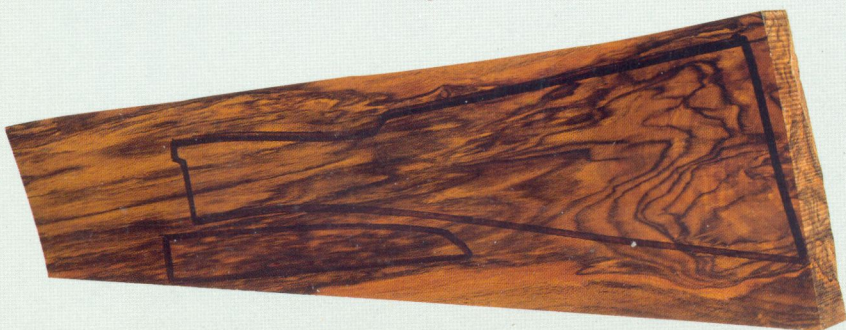
Walnut, seasoned for up to ten years, will provide the stock for the gun
